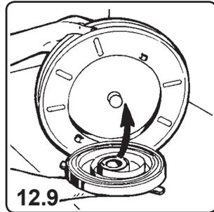
12.9) Put the drum straight and place the new spring housing centre with the utmost care. Block the tangs.
