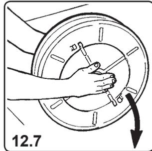
12.7) Turn upside down the drum and take out the spring housing centre paying the greatest care so that the spring does not go out of it.
