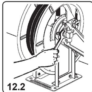
12.2) Loosen the swivel joint
