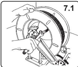
**The hose reels without hose are supplied with the unloaded spring.**
